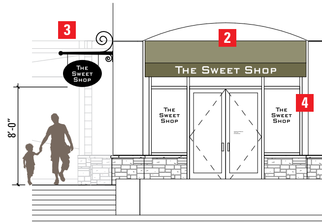
Blade Mounted Primary Identification (typ) Shown with Tenant Window Sign Scale: nts
